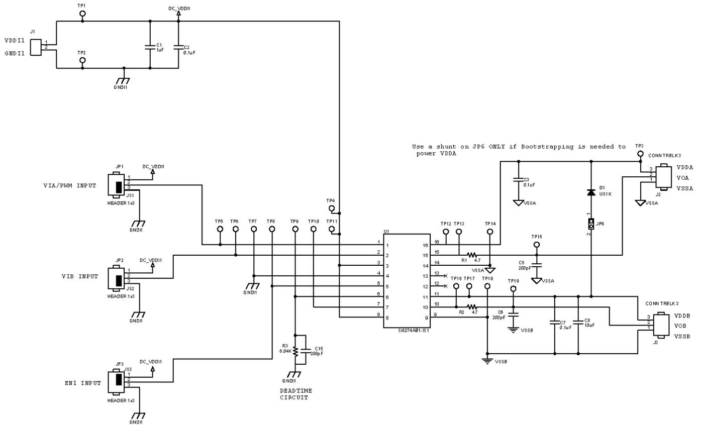
Figure 4.1. Si827x Evaluation Board Schematic (1 of 2)
