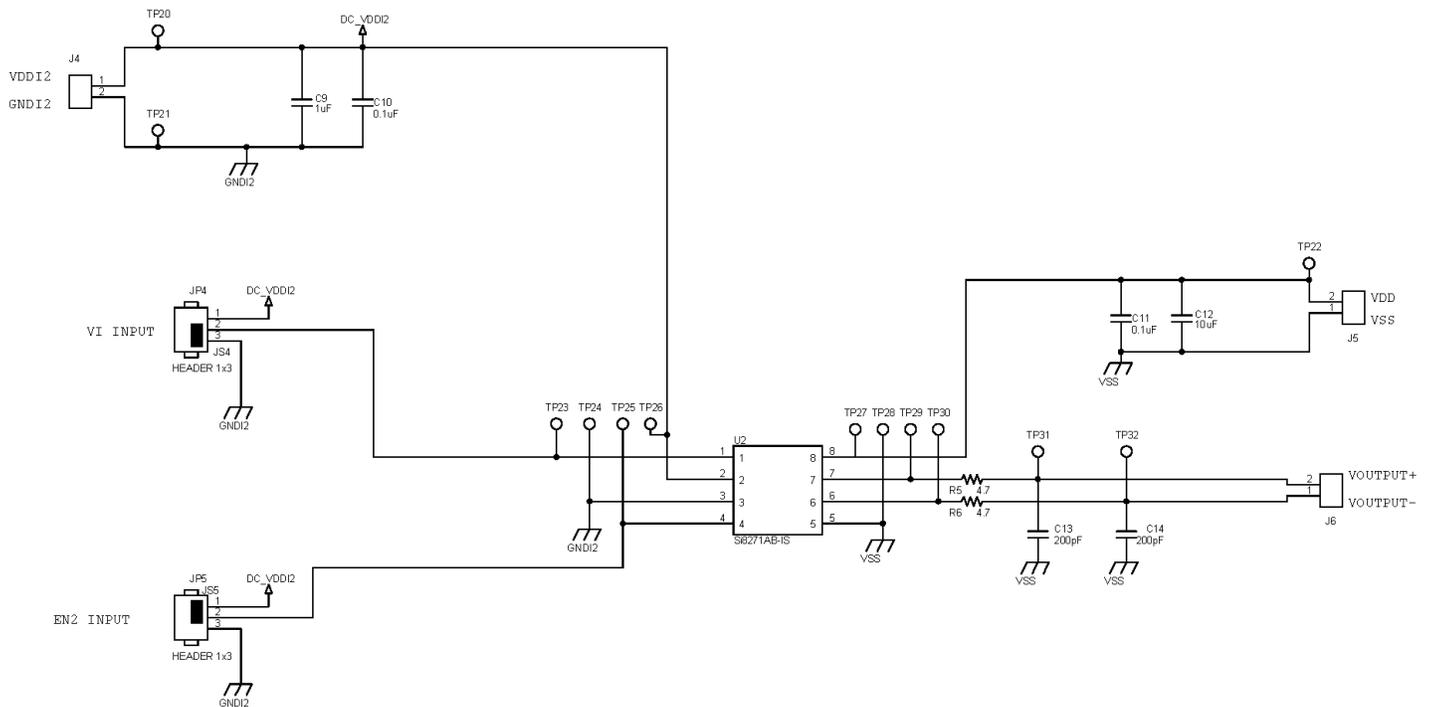
Figure 4.2. Si827x Evaluation Board Schematic (2 of 2)
