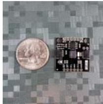
**Qwiic Visible Spectral Sensor
