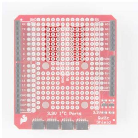
There are also buses for ground, 5V and 3.3V on the shield for Arduino outlined below.
