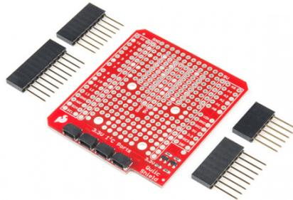
**SparkFun Qwiic Shield for Arduino**
