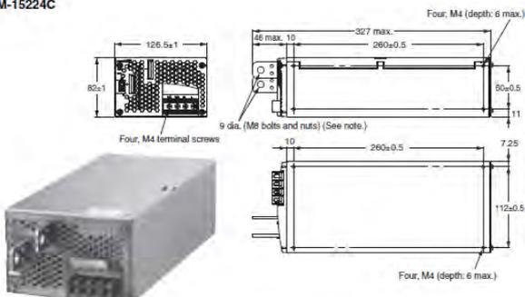
**Note:** M8 bolts and nuts for the output terminals are not included.
