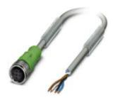
Sensor/actuator cable, 4-position, PUR halogen-free, resistant to welding sparks, highly flexible, gray RAL 7001, free cable end, on Socket straight M12, A-coded, cable length: 5 m, for robots and drag chains
