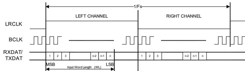
**Figure 4-43. Left-Justified Data Format (Assuming n-Bit Word Length)**
