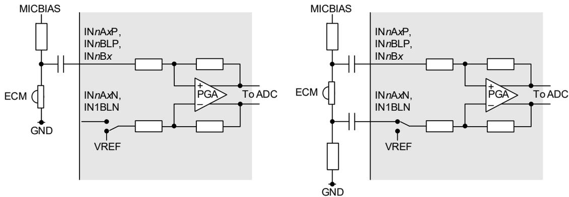
**Figure 5-2. Single-Ended and Differential Analog Microphone Connections**
