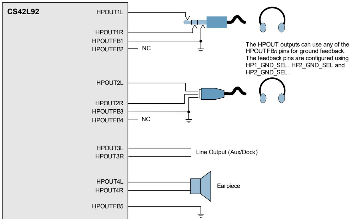
Each headphone output can support stereo (single-ended) or mono (differential) output. The illustration shows the configuration for a typical application.
