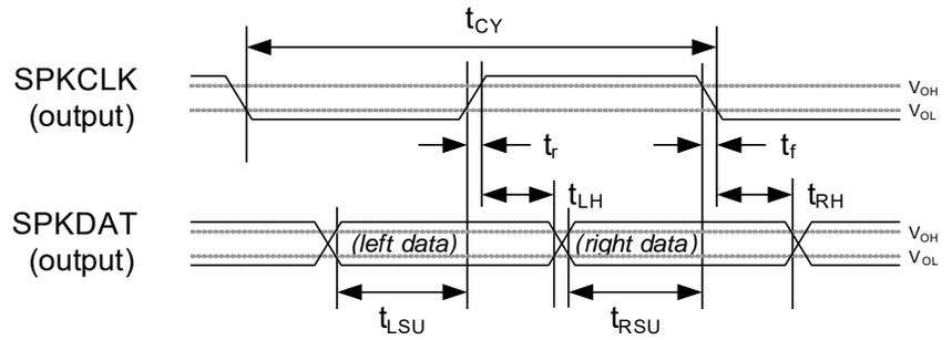
2. Digital speaker (PDM) interface timing—Mode B
