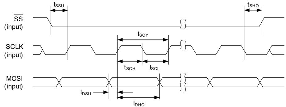
**2. Control interface timing—SPI Mode (read cycle)**
