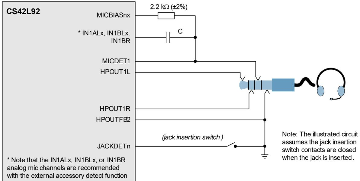
**Figure 4-57. Jack Detect and External Accessory Connections**
