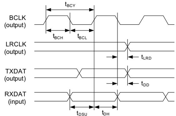
2. The timing of the AIFnLRCLK signal is selectable. If the LRCLK advance option is enabled, the LRCLK transition is timed relative to the preceding BCLK edge. Under the required condition that BCLK is inverted in this case, the LRCLK transition is still timed relative to the falling BCLK edge.
