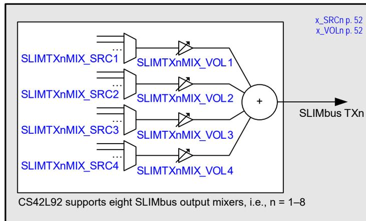
**Figure 4-19. Digital-Core SLIMbus Outputs**
