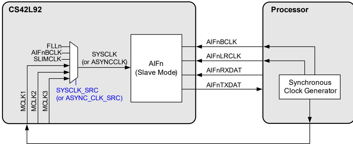
**Figure 5-13. AIF Slave Mode, Using MCLK as Reference**
