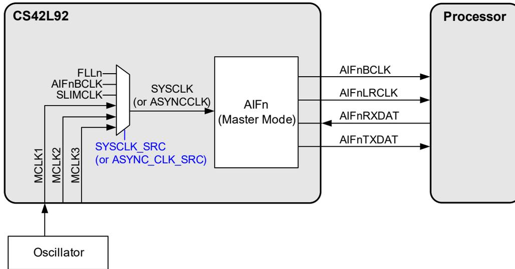
**Figure 5-9. AIF Master Mode, Using MCLK as Reference**
