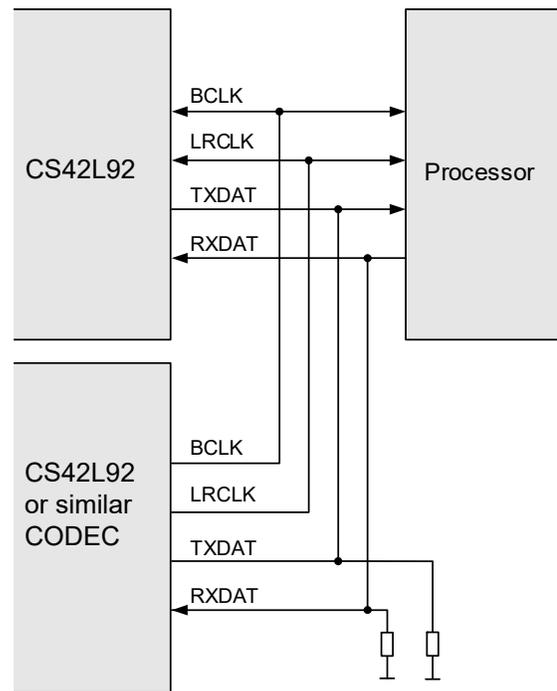
**Figure 4-49. TDM with Other Codec as Master**
