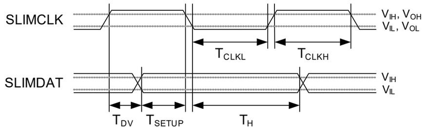
$V_{IL}, V_{IH}$  are the 35%/65% levels of the respective inputs
