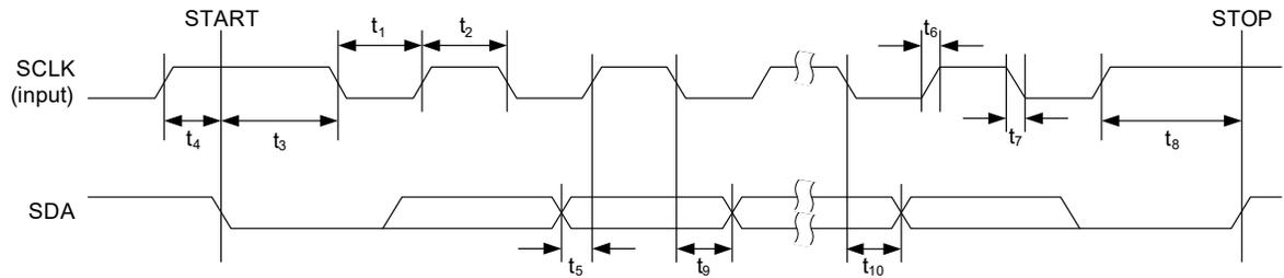
**Table 3-20. Control Interface Timing—Four-Wire (SPI) Mode**
