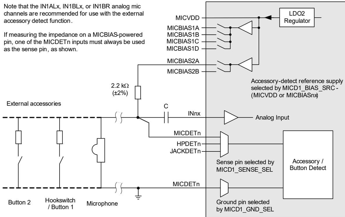
**Figure 4-61. Microphone- and Accessory-Detect Interface**
