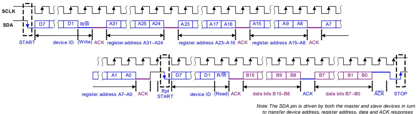
**Figure 4-70. Control Interface I<sup>2</sup>C Register Read (16-Bit Data Words)**
