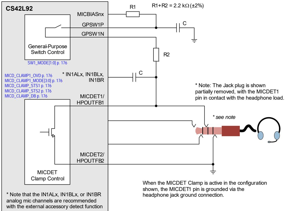
**Figure 4-60. General-Purpose Switch Circuit**
