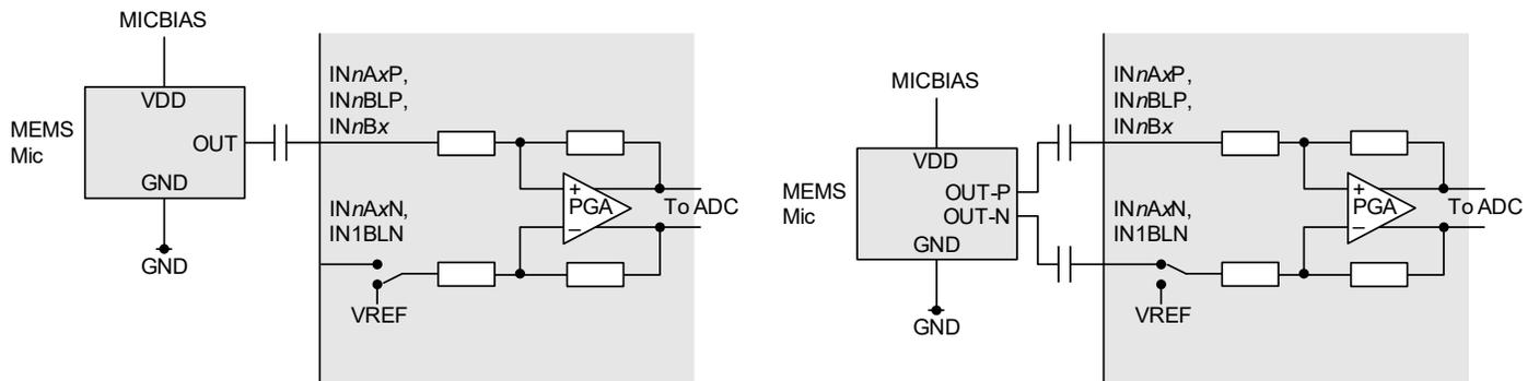
**Figure 5-3. Single-Ended and Differential Analog Microphone Connections**
