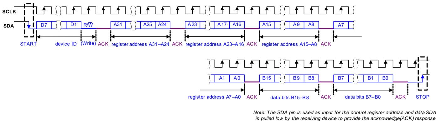
**Figure 4-69. Control Interface I<sup>2</sup>C Register Write (16-Bit Data Words)**
