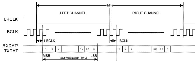
**Figure 4-42. I<sup>2</sup>S Data Format (Assuming n-Bit Word Length)**
