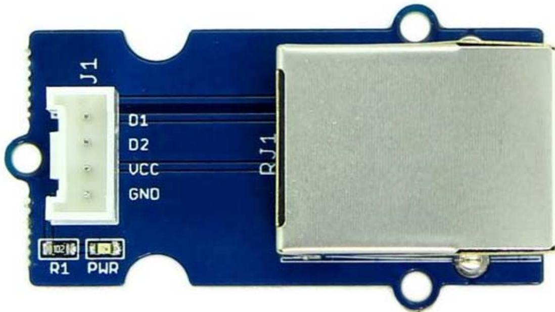
The Grove-RJ45 Adapter is a module which can convert a standard Grove connector to a RJ45 connector. Universal 4-Pin Grove cables can not meet the requirements when Arduino remote connect and control Grove module. Through two RJ45 adapter and a cable, It is able to achieve communication between Arduino and Grove module. This help solve the problem that Arduino and Grove are not convenient to connect because of the distance issue.
