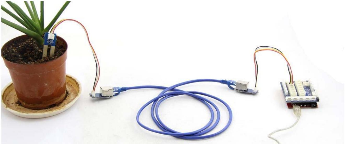
You may need to write the code by yourself for the special applications. But we can guarantee that you can always know the soil moisture of plants by observing the output data of the moisture sensor.
