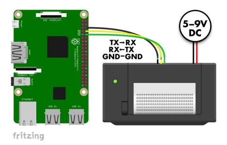
Really you can use any GND shown in the pinout diagram above. The third pin is easy to locate, but that spot's sometimes occupied by other hardware like small cooling fans.
