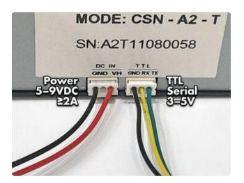
The Mini thermal printer has two 3-pin sockets—one for power, one for serial communication. Power goes to the jack labeled "DC IN." Only the outer two pins of this connector are used.
