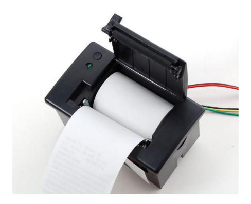
As described on prior page, power the printer using a 5V to 9V 2A or higher power supply, such as wiring up a 2.1mm DC power jack:
