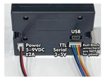
The Tiny printer has three sockets: a 2-pin connector for power, 5-pin for TTL serial communication, and a USB port.
