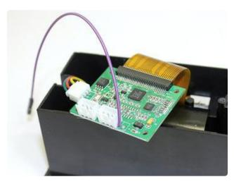
Solder the wire to the DTR pad. Top, bottom, doesn't matter...it's right up against the serial connection plug, so use whatever path works best for you, there's ample room for routing the wire around either way.
