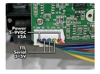
The Nano printer and "printer guts" have a single 5-pin connector for power and serial data. The outermost red and black wires are for +V and ground, following typical conventions.
