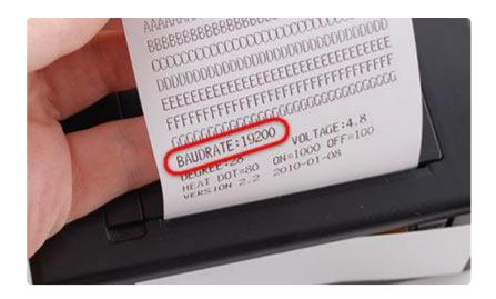
If no baud rate is shown, or your printer has no self-test page feature, first assume 9600 as the default. In that doesn't work in tests that follow, then try 19200.
