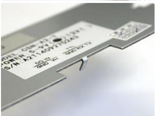
On the back plate, there's a small metal "finger" between the serial and power sockets. Using pliers, this can be bent back to provide an exit route for the DTR wire.
