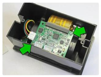
Take the back plate off, then remove the two (or sometimes four) Phillips screws holding the circuit board in place.
