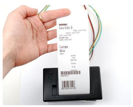
If this does not work, first check that the printer and Arduino are both powered, and that the data in, out and ground wires are properly connected to the Arduino.
