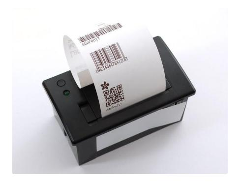
Add printing to any microcontroller project with these very cute thermal printers. Also known as receipt printers, they're what you see at the ATM or grocery store. Now you can embed a little printer of your own into a project. These printers is ideal for interfacing with a microcontroller, you simply need a 3.3V to 5V TTL serial output from your microcontroller to print text, barcodes, bitmap graphics, even a QR code!
