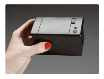
Our Mini Thermal Receipt Printer () is a popular choice as it accommodates a full-length thermal roll (15m/50') (), meaning fewer paper changes. It's also available in a starter pack () that includes a 5V power supply and DC jack adapter.
