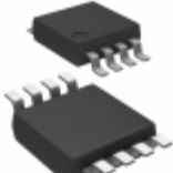
MCP4552T-502E/MS Microchip Technology IC POT DGTL 5K SGL 8-MSOP
