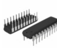
PIC16F527-E/P Microchip Technology IC MCU 8BIT 1.5KB FLASH 20DIP
