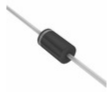
1N6267-E3/73 Vishay Semiconductor Diodes Division TVS DIODE 5.5VWM 10.8VC 1.5KE
