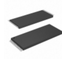
AT29C040A-10TI Microchip Technology IC FLASH 4MBIT 100NS 32TSOP
