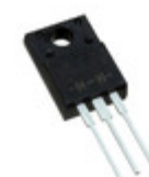
TSF40H200C COG TSC (Taiwan Semiconductor) DIODE ARRAY SCHOTT 200V ITO220AB
