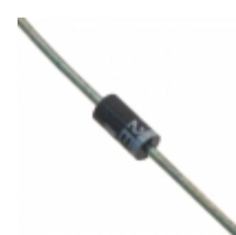
3EZ5.6D10E3/TR8 Microsemi Corporation DIODE ZENER 5.6V 3W DO204AL
