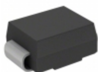
CZRB5350B-HF Comchip Technology DIODE ZENER 13V 5W SMB
