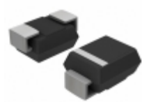
SMLJ45CA-TP Micro Commercial Co TVS DIODE 45VWM 72.7VC SMC
